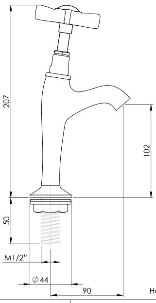
Holes to be drilled: 30 mm
